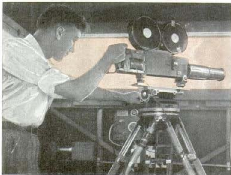
Complete time and space record of plane landings and takeoffs is filmed, 3 exposures per second, from hut on Wright Field
